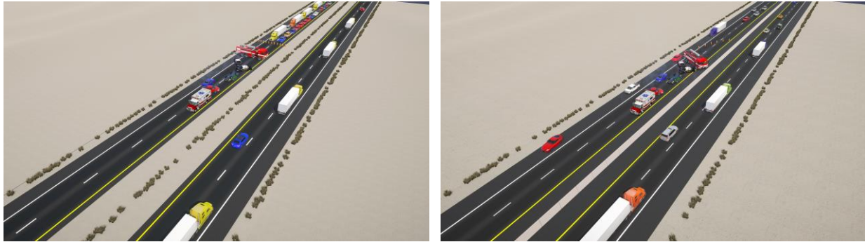
The existing I-40 configuration is shown on the left. The proposed I-40 configuration on the right shows how the wider 12-foot shoulders could be used to get traffic moving if lane closures are needed to respond to incidents.
