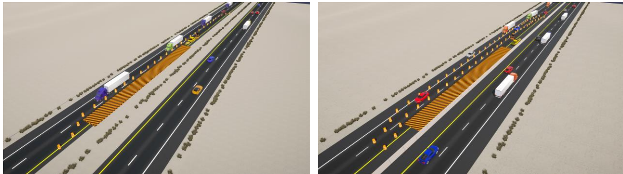
The existing I-40 configuration is shown on the left. The proposed I-40 configuration on the right shows how the wider 12-foot shoulders could be used to maintain 2 lanes on I-40 during maintenance activities
