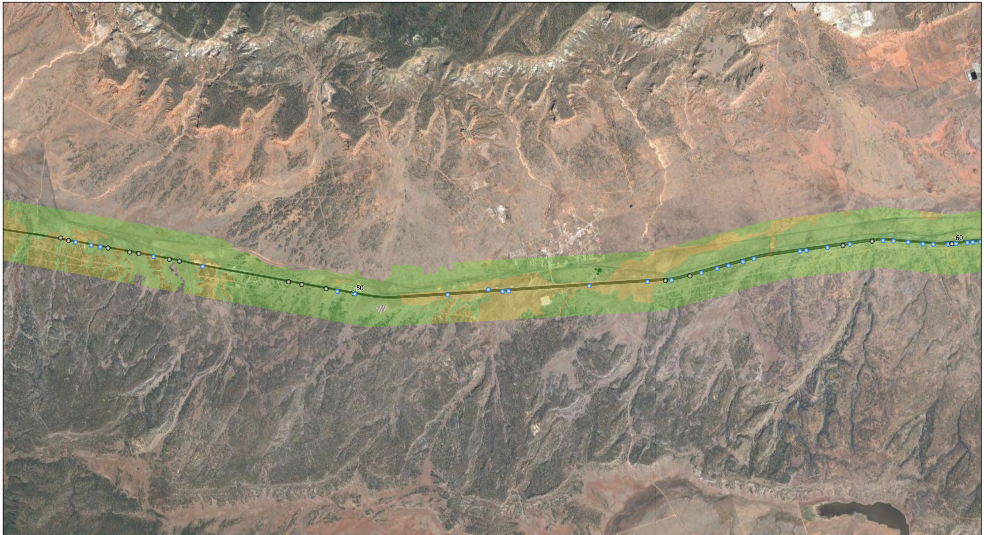
Exhibit 4 - I-40 Soil Corrosion Potential - Concrete Milepost 45 - 60
