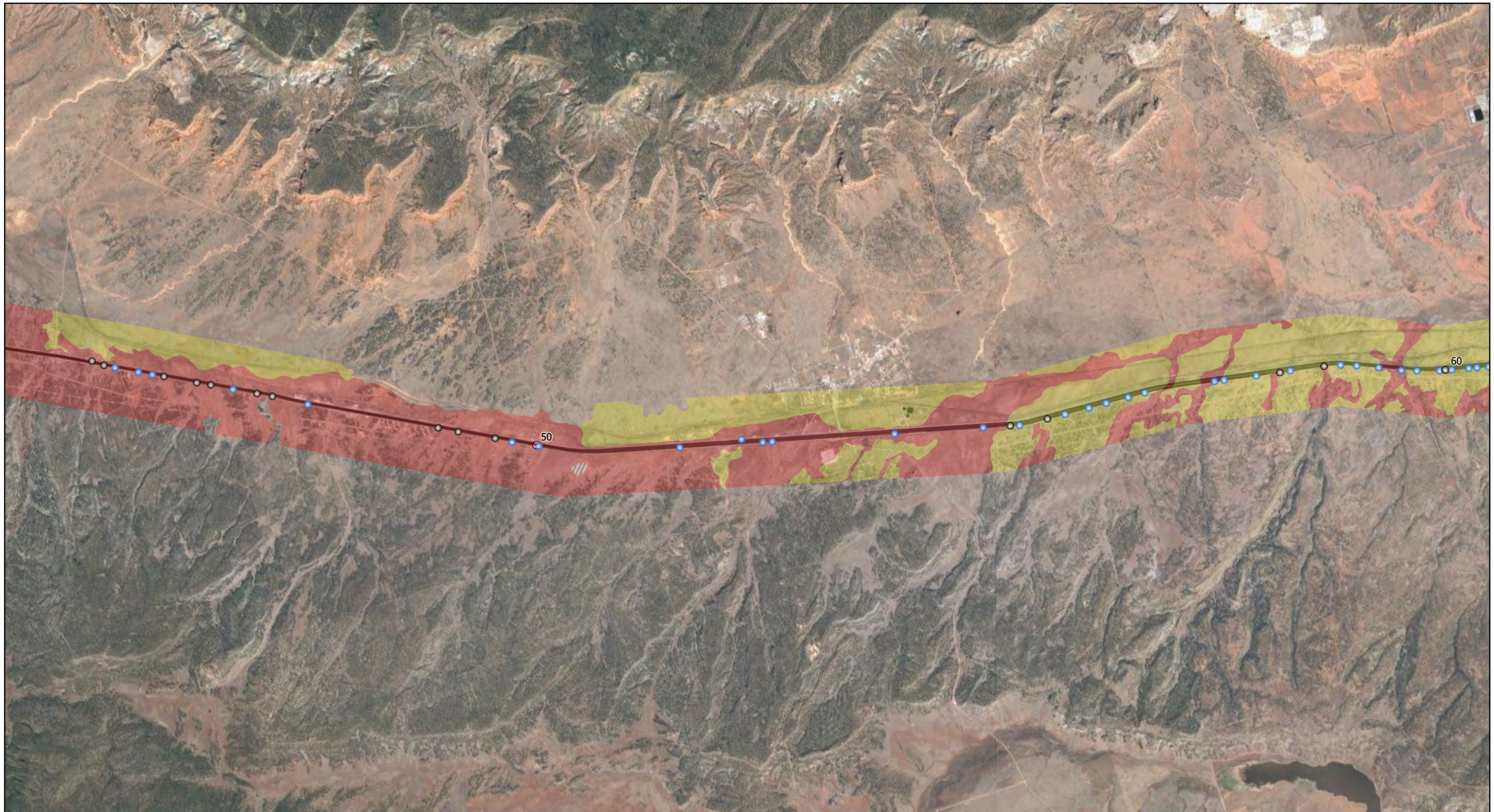
Exhibit 14 - I-40 Soil Corrosion Potential - Steel Milepost 45 - 60
