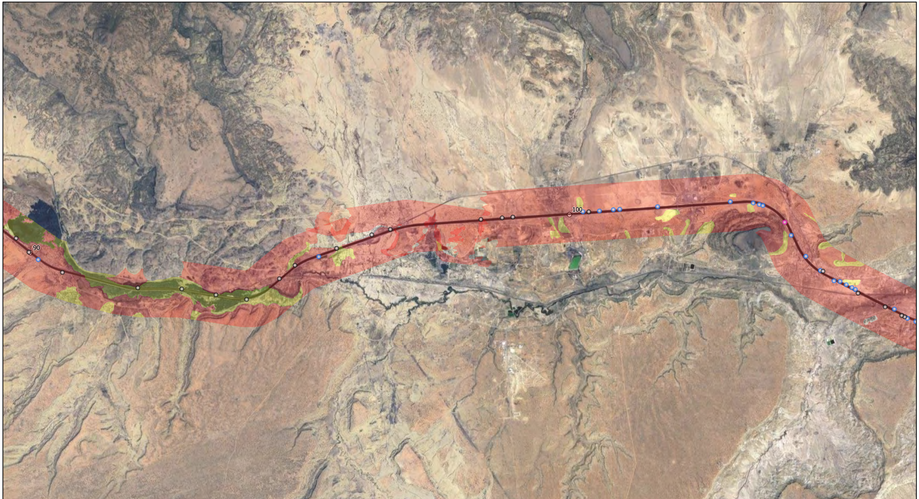
Exhibit 17 - I-40 Soil Corrosion Potential - Steel Milepost 90 - 105
