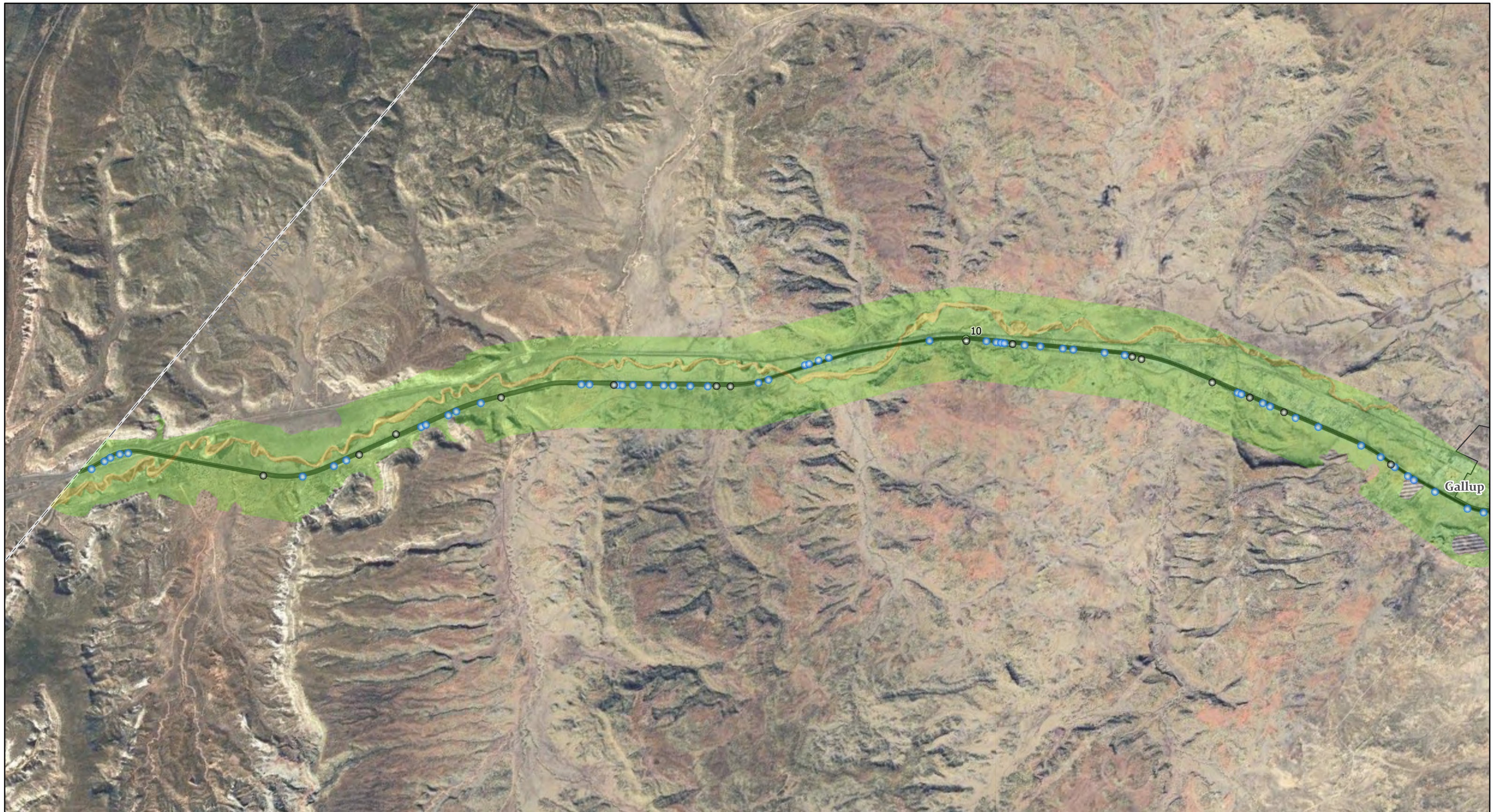
Exhibit 1 - I-40 Soil Corrosion Potential - Concrete Milepost 1 - 15
