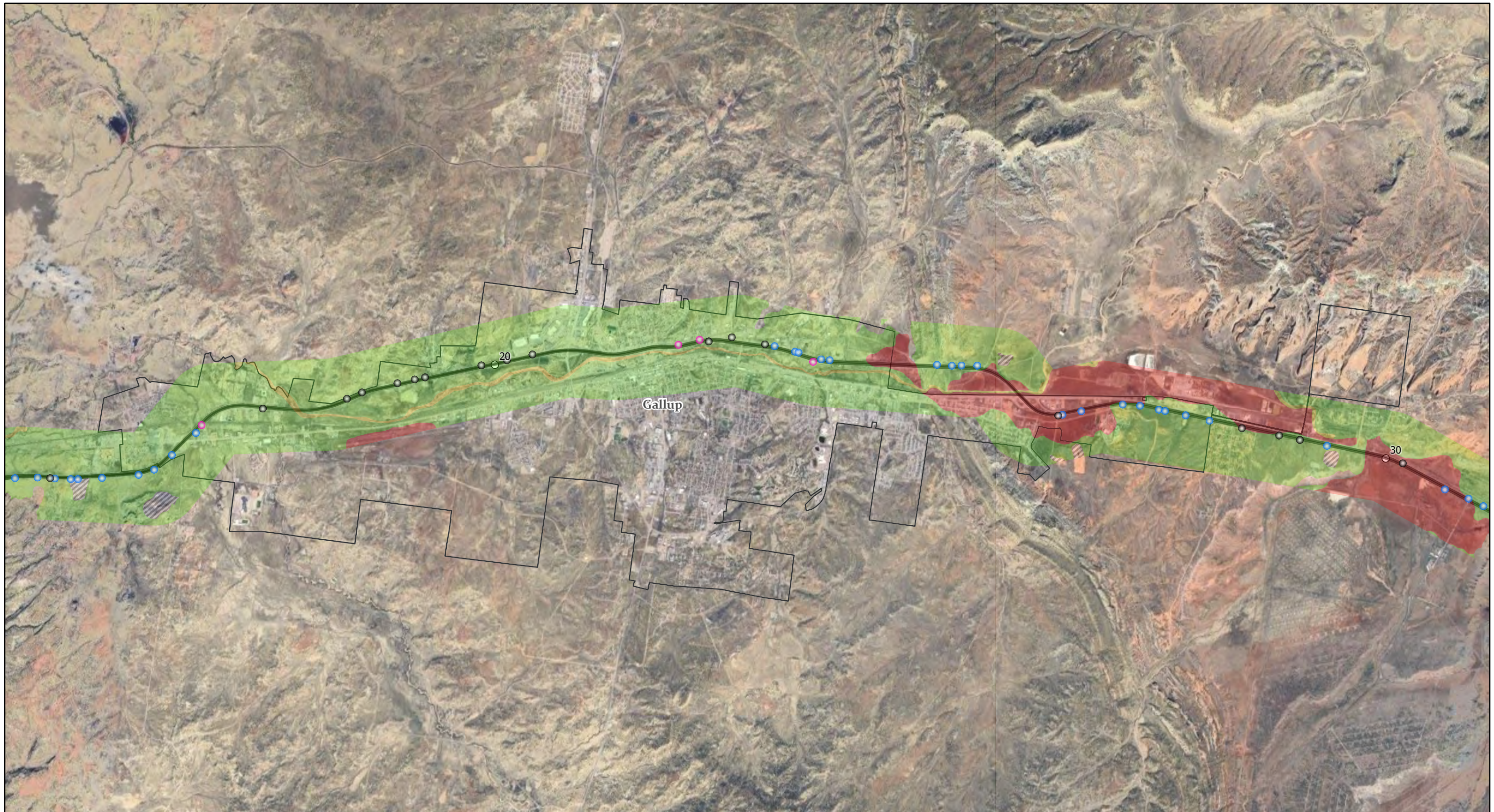
Exhibit 2 - I-40 Soil Corrosion Potential - Concrete Milepost 15 - 30
