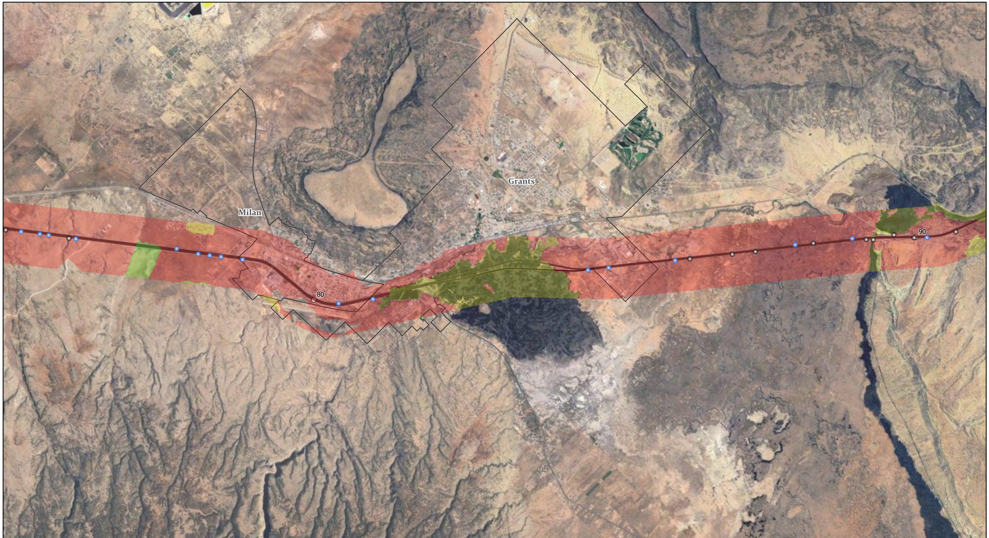
Exhibit 16 - I-40 Soil Corrosion Potential - Steel Milepost 75 - 90
