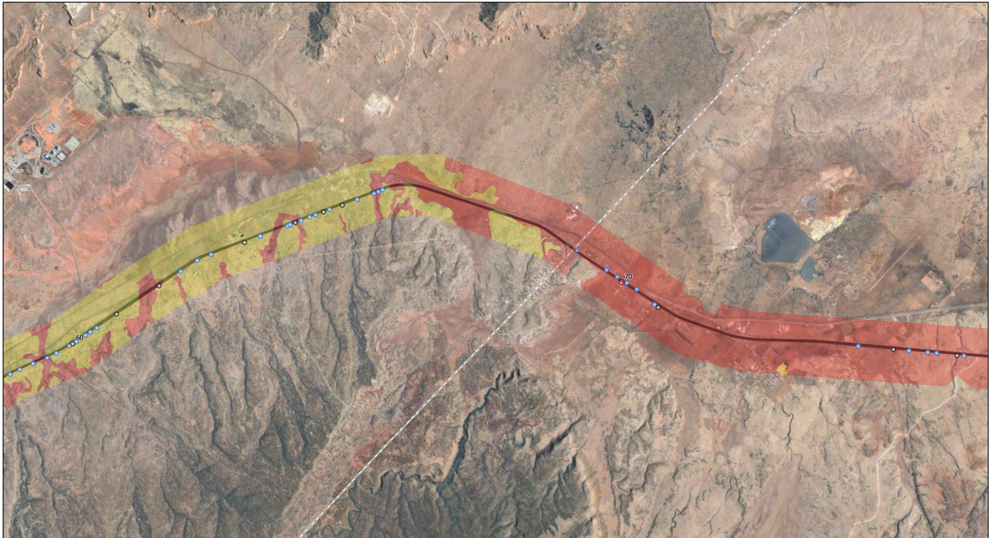
Exhibit 15 - I-40 Soil Corrosion Potential - Steel Milepost 60 - 75
