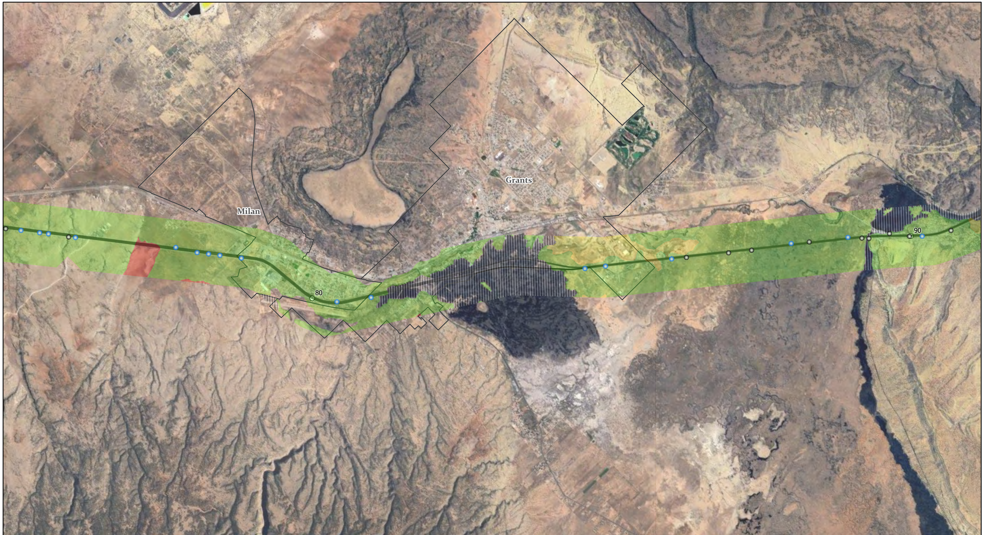
Exhibit 6 - I-40 Soil Corrosion Potential - Concrete Milepost 75 - 90
