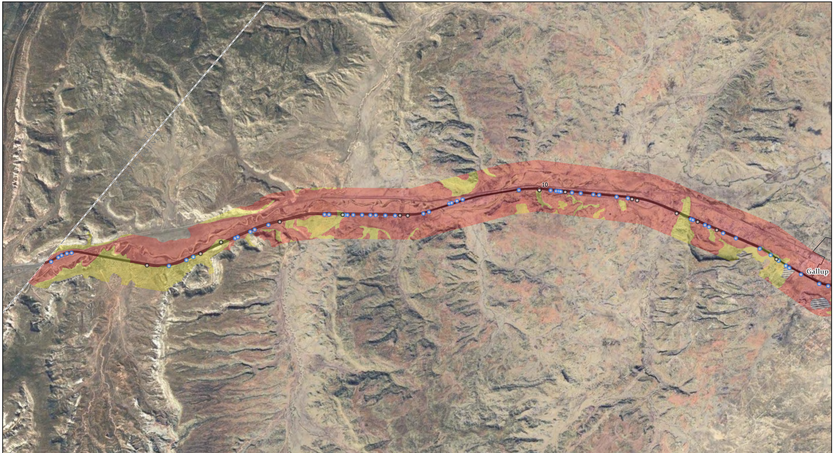
Exhibit 11 - I-40 Soil Corrosion Potential - Steel Milepost 1 - 15
