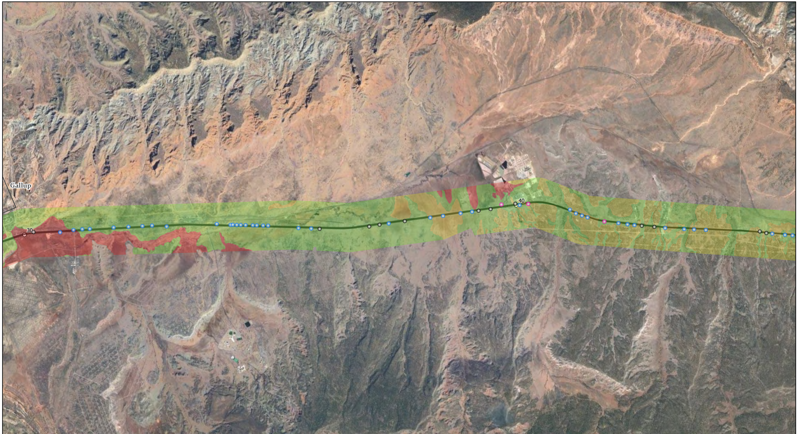
Exhibit 3 - I-40 Soil Corrosion Potential - Concrete Milepost 30 - 45
