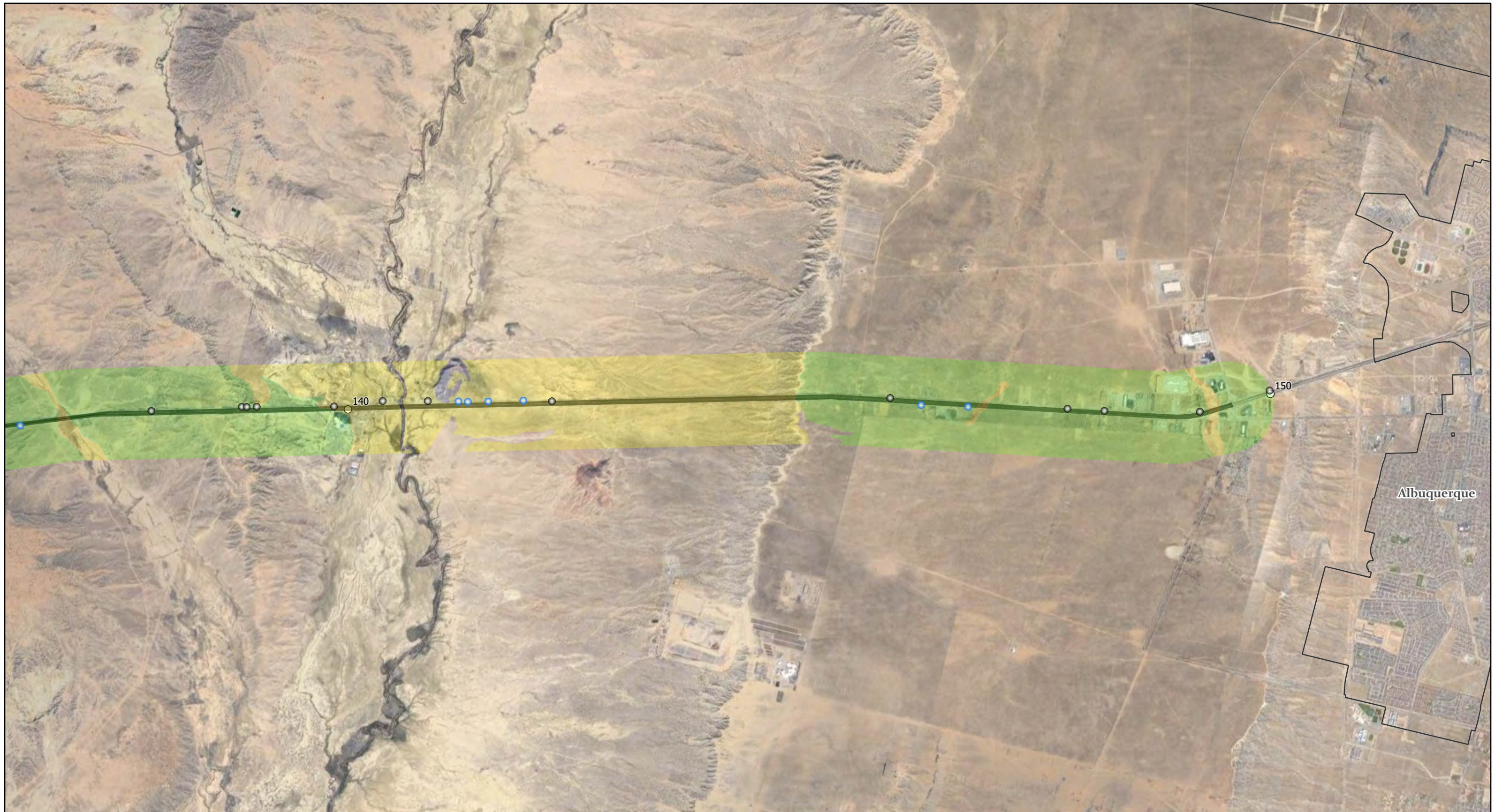
Exhibit 10 - I-40 Soil Corrosion Potential - Concrete Milepost 135 - 150
