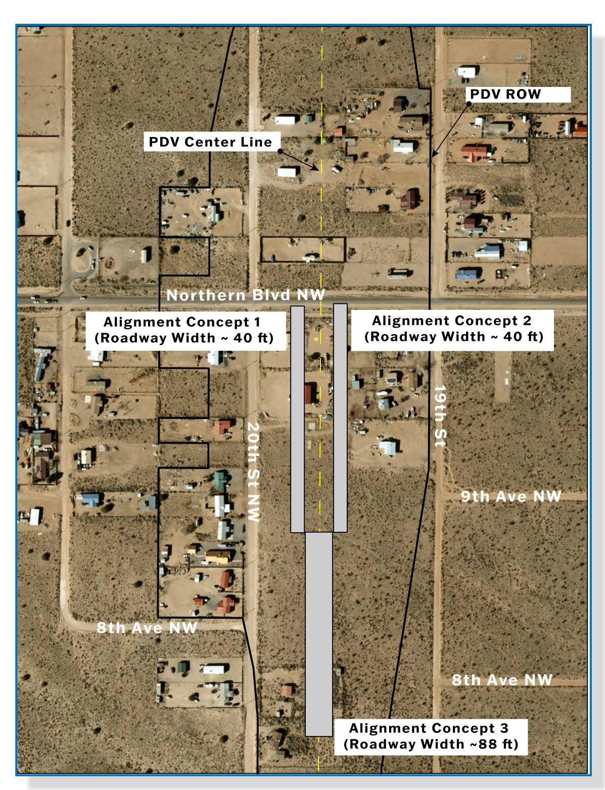
**ALIGNMENT OPTION 3.** Center with Depressed Median - 2-lane road with shoulders and a depressed median in the center of the corridor. Shoulder to shoulder width of this roadway is 88 ft.
