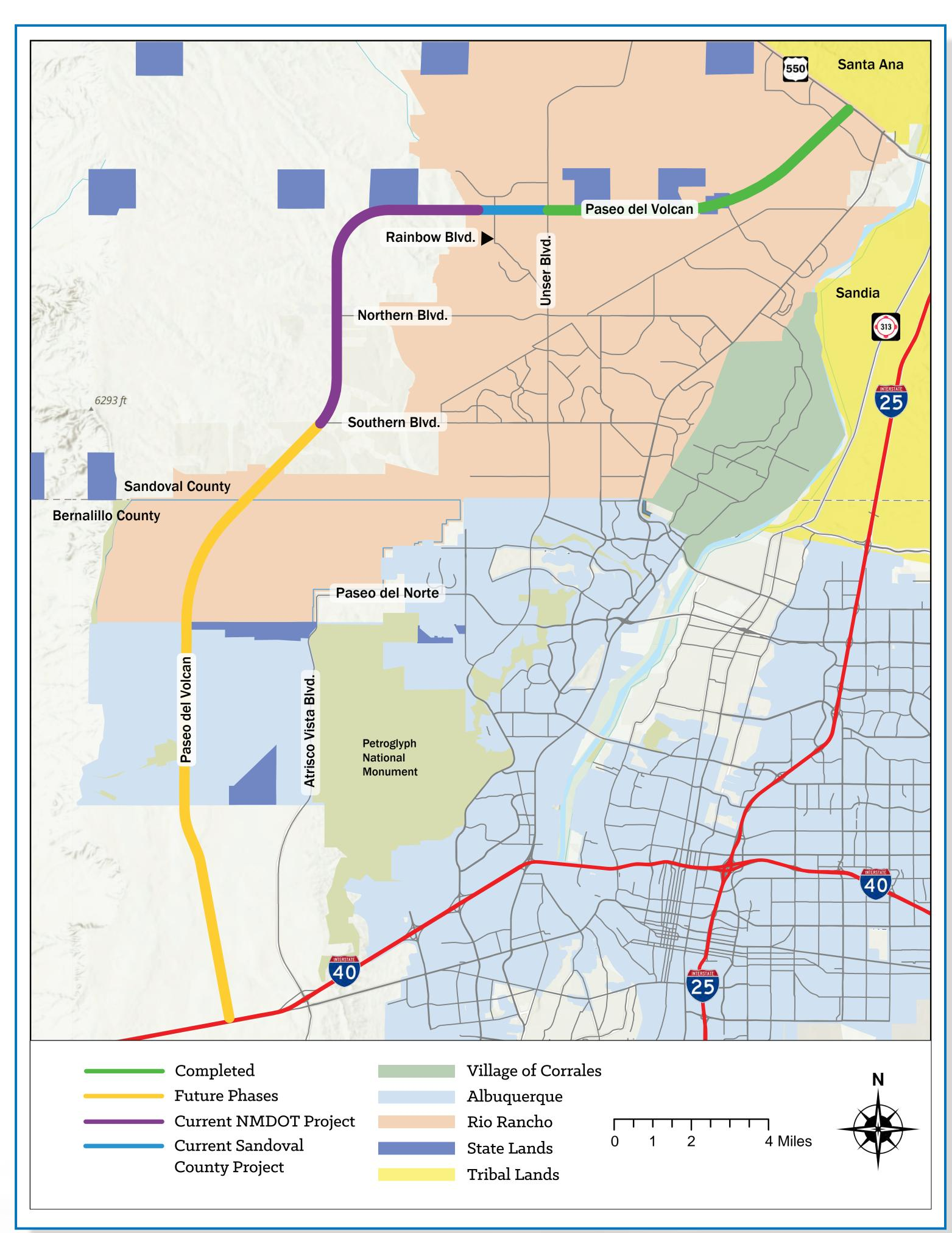
The EIS authorized right-of-way acquisition for a corridor along the alignment identified and the design development of a 2-lane limited access road. The northern 7 miles has been constructed leaving an additional 22 miles to complete the connection to I-40.
