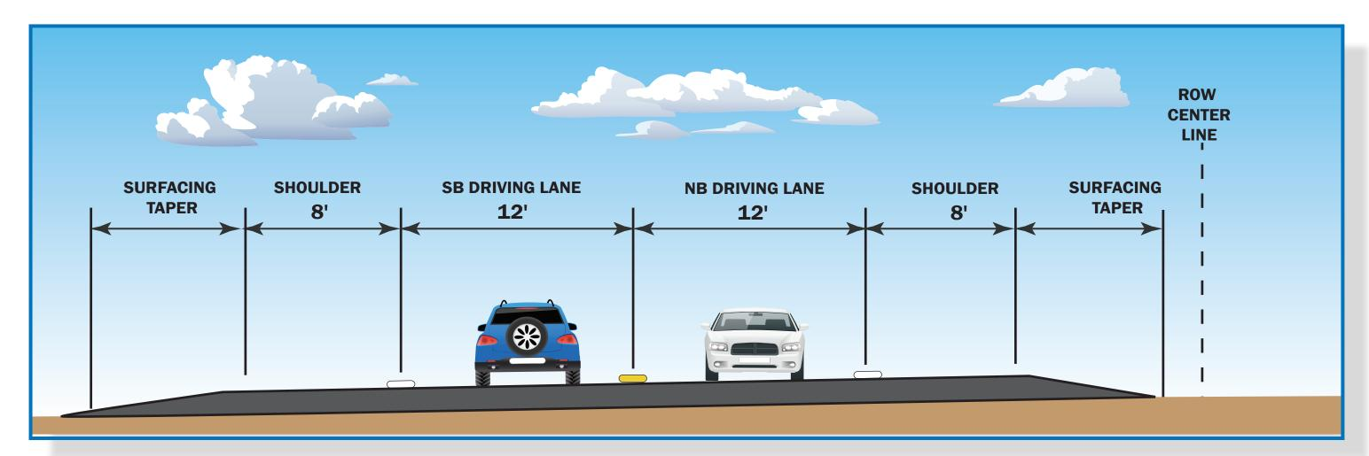
ALIGNMENT CONCEPT 2. East (right) Offset - the 2-lane road with shoulders on the east side of the corridor centerline. Shoulder to shoulder width of this roadway is 40 ft.
