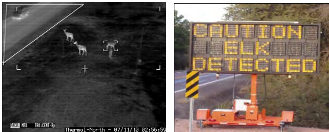
Figure 7-10. Example of thermal target acquisition software used to activate motorist alert signs (left) and sign activated when a target is identified as wildlife large enough to pose a safety concern to motorists.
