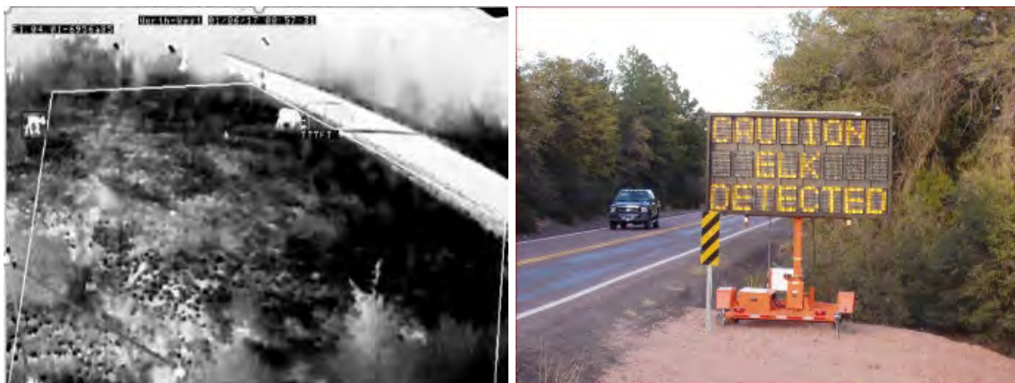
Figure D-56. Screen capture of thermal camera image of elk cow and calf and motorist warning sign on Arizona SR 260 (photo credit: AZGFD and CrossTek, LLC).
