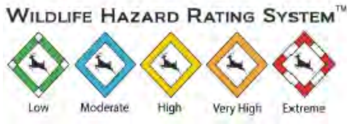
Figure D-50. Variations of deer-vehicle collision warning signs with flashing border intended to alert motorists during peak potential crash periods. color and flash pattern can be changed as needed (from Sielecki, 2017).
