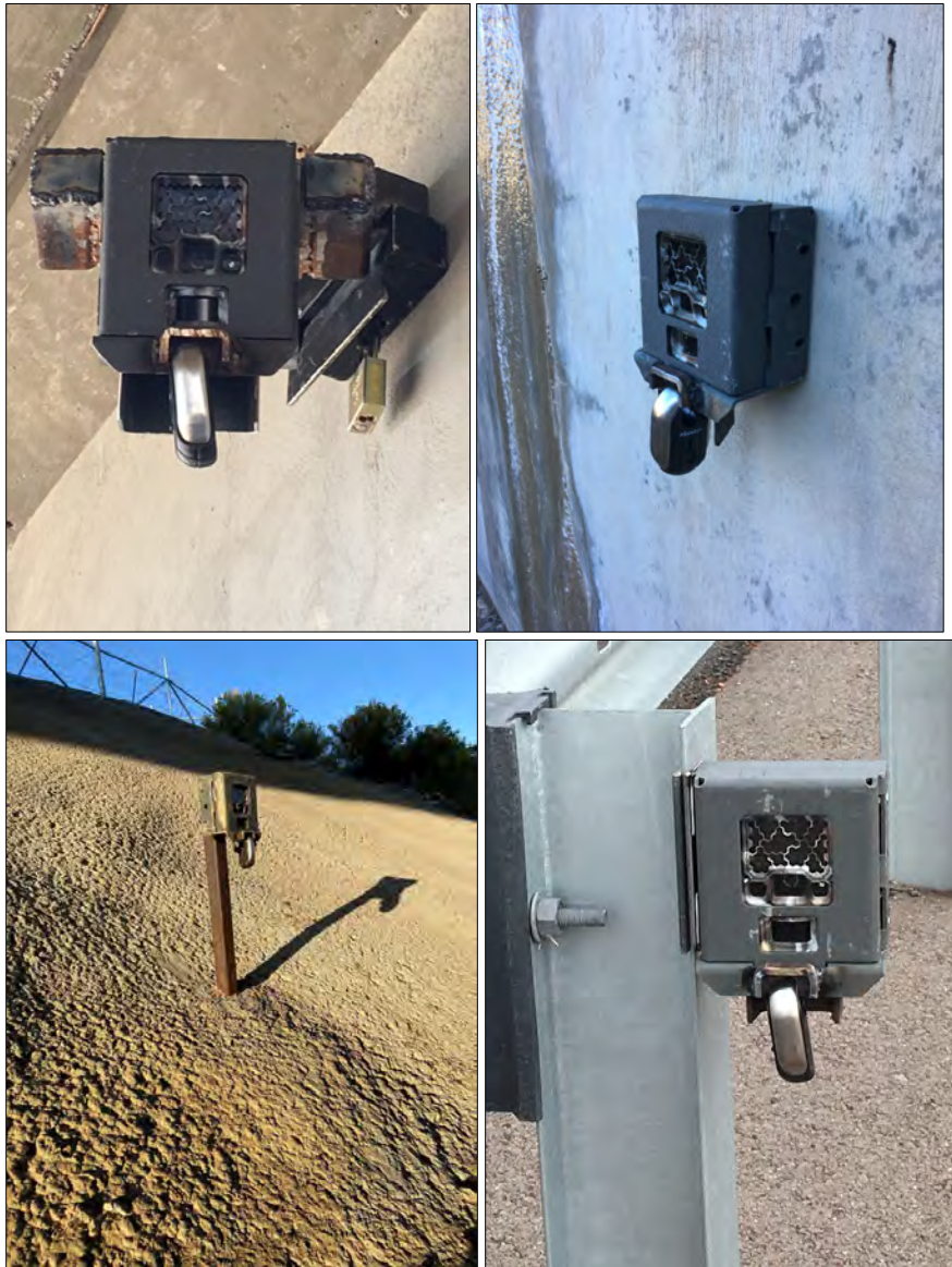
Figure 7-13. Consistent data collection from cameras is important to determine mitigation success, and taking measures to secure cameras is essential. Options like these being used in New Mexico can help reduce theft, and include articulated mounts that deter cutting with power or hand tools (upper left), flush mounts with robust anchors to hinder prying (upper right), cameras welded to poles and set in concrete (lower left), and hiding cameras in discrete locations such as behind a guardrail (lower right).
