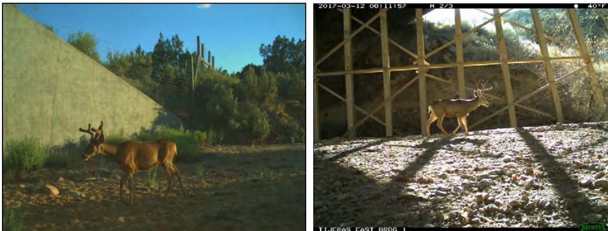
Figure 7-8. Example of adequate monitoring at a small culvert (left) and at a larger road-crossing structure (right) in New Mexico using motion-triggered, remote cameras. The cameras capture both approaches and crossings of deer and other wildlife at the culvert, allowing for the calculation of passage rates, thus contributing to knowledge about the effectiveness of mitigation measures. At the larger structure, most approaches are expected to result in the successful passage of wildlife, at the same time that documenting all approaches is logistically more difficult; the use of cameras is more geared toward documenting the number of passages and the full range of species using the structure (right).
